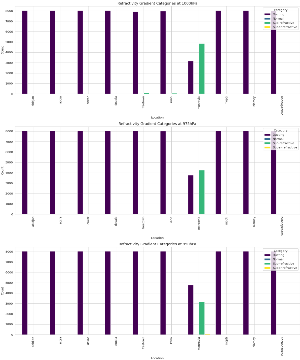
Figure 10: Statistical distribution of refractivity gradients across all study locations, highlighting dominant propagation conditions
